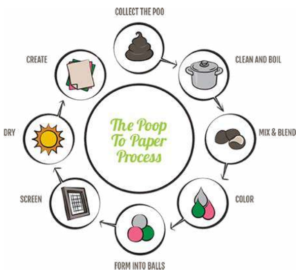
Paper production process from cow dung (Source: NET)
