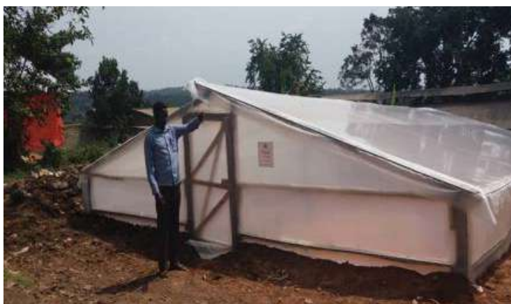
Drying poultry waste in a solar dryer (Task Farm, Rubaga, Tel: 0782747326)
